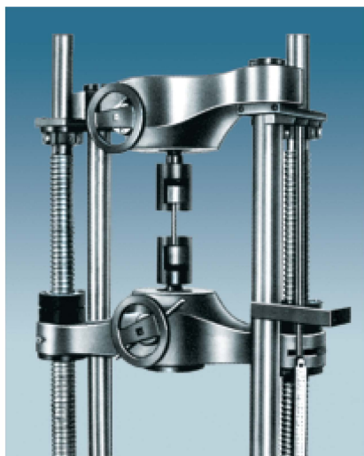
ATTACHMENT FOR TENSION TEST FOR SHOULDERED AND THREADED SPECIMENS
