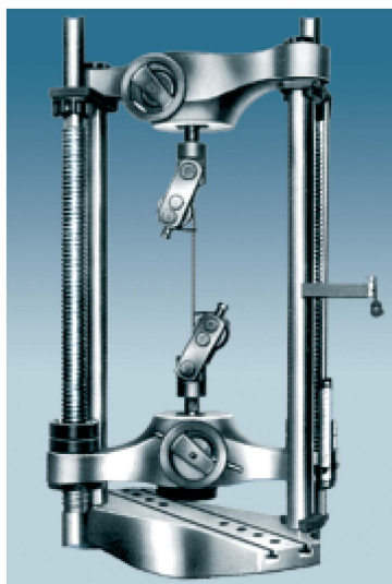
ATTACHMENT FOR TENSION TEST FOR WIRE ROPES
