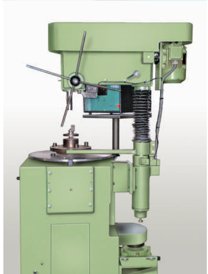
Vertical Single Plane machine with Optional Vertical or Horizontal Drill Head Attachment.
